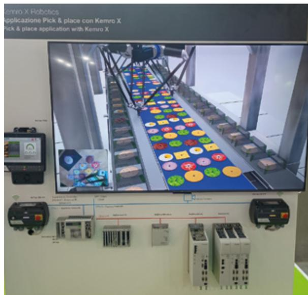
*manage a wide range of solutions. A perfect example of coordination in material flow is represented by Keba pick & place application, the result of a technologies mix such as machine vision, applied AI for image processing and digital twin. This solution was divided into two parts: a physical one consisting of one Delta and one camera, and a virtual one composed of four Deltas, three conveyor belts and a camera.*
