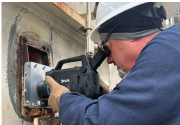
*Essential is the integration of FLIR's Thermal Studio Pro software: with the Route Creator tool, inspections are no longer reactive they're pre-planned and executed with precision. Technicians follow a defined route with inspection points loaded into the camera, eliminating guesswork and ensuring consistency. After inspections, images are automatically organized by inspection point, and reports are generated in minutes using professional templates.*
